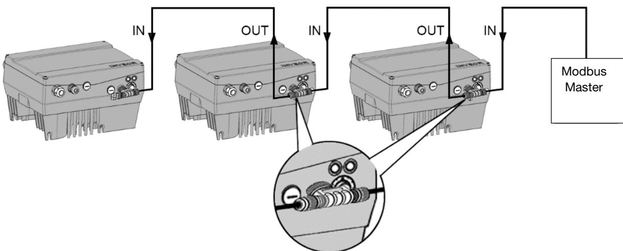
Fig.: 1 Wiring and bus connection
