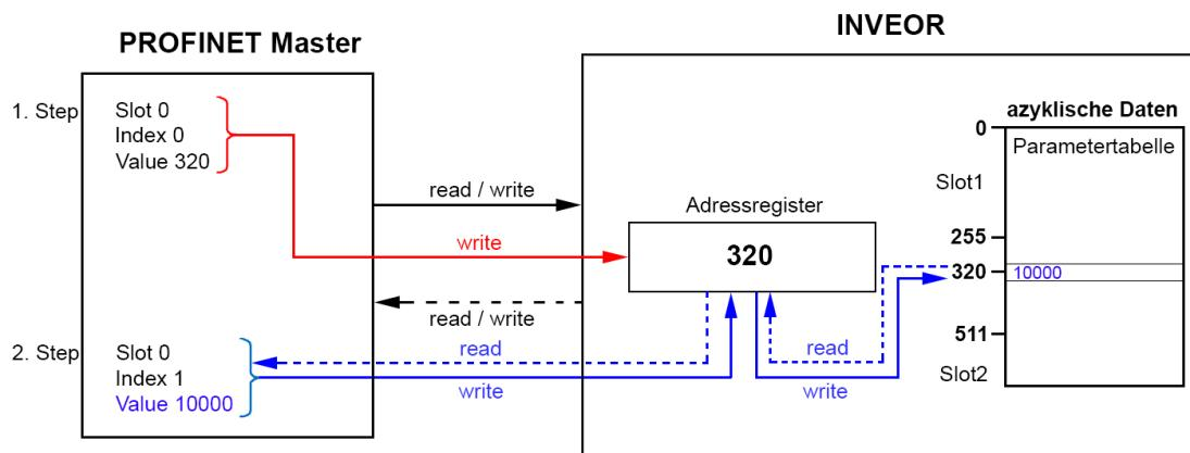
In the first step, a value 0 - 511\* must be written into the address directory of the INVEOR by the PROFINET master via slot "0", index "0".
