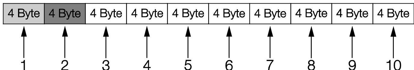
The first two process variables (status word and actual frequency) cannot be parameterised and are always sent. The remaining 8 process variables can be configured using parameters [6.080](#) to [6.087](#).
