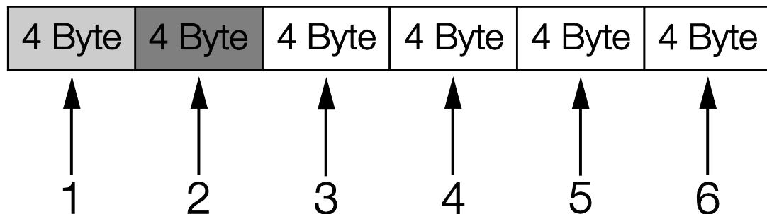
The first two process variables (control word and target value) cannot be parameterised and are always expected. The remaining 4 process variables can be configured using parameters 6.110 to 6.113.
