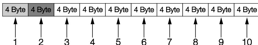
The first two process variables (status word and actual frequency) cannot be parameterised and are always sent. The remaining 8 process variables can be configured using parameters [6.080](#) to [6.087](#).
