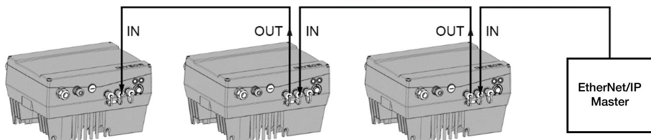
Fig.: 4 Wiring and bus connection (Example connection INVEOR M size C)
